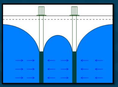
CONE OF DEPRESSION – DRAW DOWN WITH BOTH PUMPS RUNNING IN A CONFINED AQUIFER
