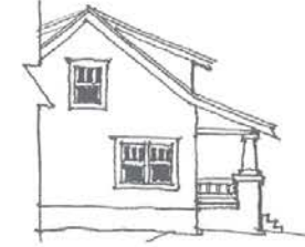
A shed-roof porch continues the line of the primary roof with a change in the slope
