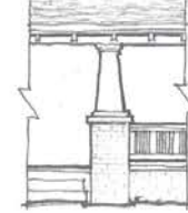
Wide tapered box column on brick base with wood railing
