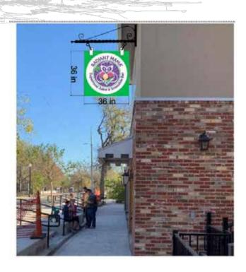
The sign will be located on a new metal bracket located towards the top of the second story. Per the Bastrop Building Block (B³) Code, a blade sign can be up to four feet in height and length but cannot be more than 6 square feet in size. The applicant has proposed the sign to be 3-foot by 3-foot square, but the sign can be scaled to meet the requirements and maintain the look of the sign.
