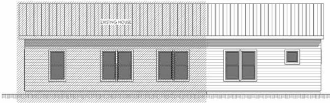
The new addition is to the rear of the structure and will continue the side façade. The siding, roof, and windows will all match the existing style and materials of the existing house.
