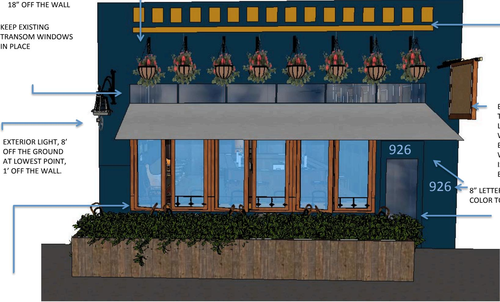
OPTION 1: This first option includes a 12' 6" Double leaf single light casement window unit (three section of double leaf casement windows mullered together into one unit). The window unit is to be constructed of Spanish cedar, putty glazed with safety glass. The hardware provided will be 18 each 3" x 3" hinges, 1 each casement sash lock per section and t2 each slide bolts per section. Each pair of sash is to be rabbeted and beaded at the meeting stile.
