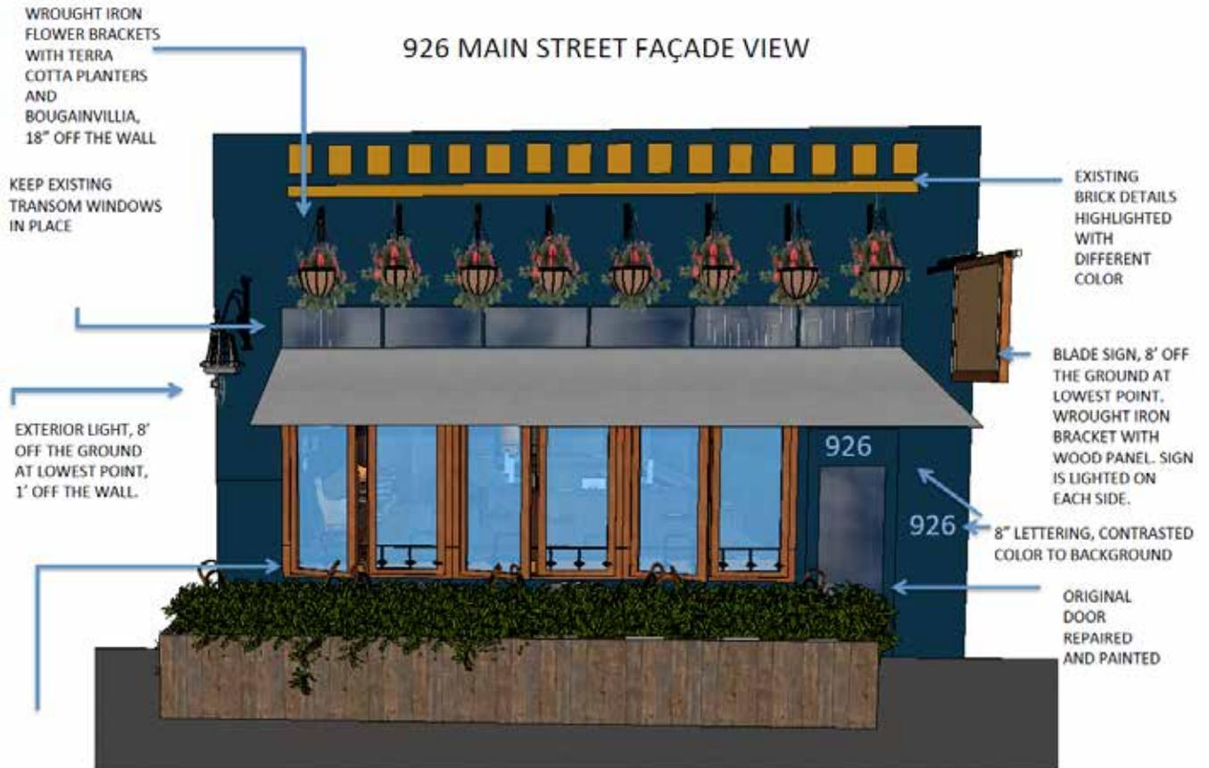
OPTION 1: This first option includes a 12' 6" Double leaf single light casement window unit (three section of double leaf casement windows milled together into one unit). The window unit is to be constructed of Spanish cedar, putty glazed with safety glass. The hardware provided will be 18 each 3" x 3" hinges, 1 each casement sash lock per section and 2 each slide bolts per section. Each pair of sash is to be rabbeted and beaded at the meeting stile.
