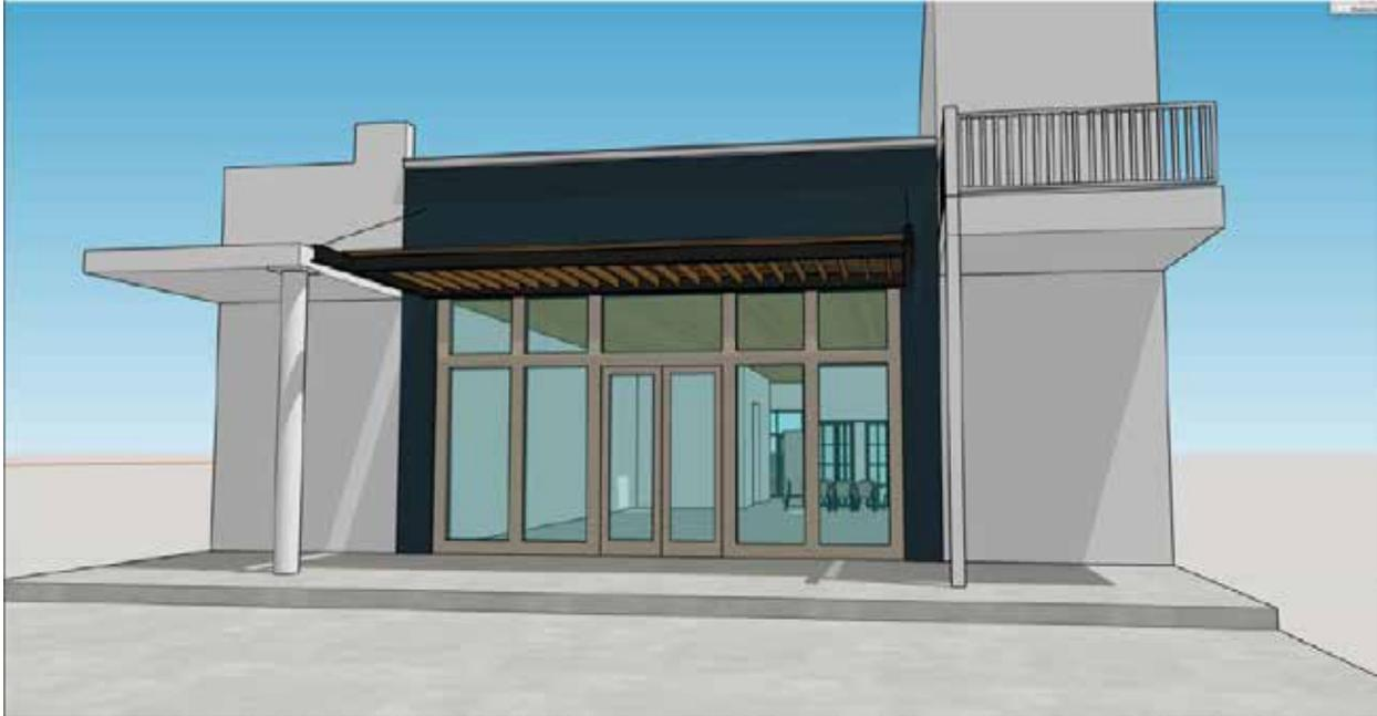
The new awning would be a steel flat awning with painted steel channels at the perimeter and stained wood infill including exposed joists. The awning will be connected with steel rod tiebacks to the stone façade (Attachment 6).
