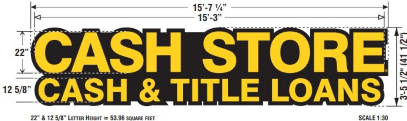
**SCOPE OF WORK: FABRICATE, SHIP AND INSTALL ONE (1) NEW LED ILLUMINATED CHANNEL LETTER SIGN TO BE RACEWAY MOUNTED.**
