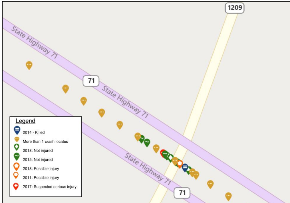
Figure 24: Collisions at FM 1209 and SH 71 Intersection, 1/1/11-7/30/19 27 (Source: CRIS) Between January 2011 and July 2019, 259 collisions occurred at the intersection of FM 1209 and SH 71. The table below displays the collisions by year and severity.
