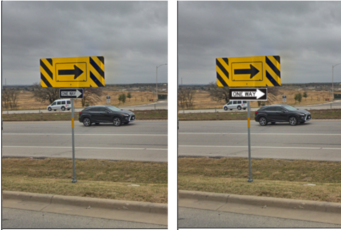
Figure 22: Left – FM 969 at SH 21 (Google Maps, 2018). Right – Artist rendition of oversized ONE-WAY sign
